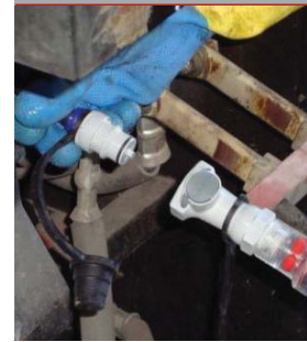
One connection waters all cells simultaneously
